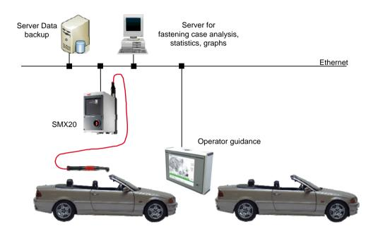
SMX20 + SMX10, connected to a customer-supplied graphic display unit
