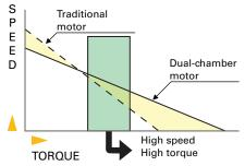
In terms of performances, the efficiency of a standard one-chamber motor is absolutely lower than a dual-chamber motor as IH wrenches.
